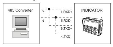
Note. RS-422 & 485 communication is optional specifications, which are supported through COM2. Refer to page 42 (Set Mode) for the setup.
