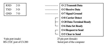
(2) COM2 - RXD: Pin No. 2, TXD: Pin No. 3, GND: Pin No. 7 (Option)
